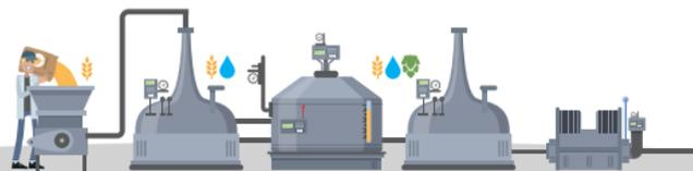
CONCASSAGE MILLING → CUISSON DU MASH MASHING → FILTRATION LAUTERING → ÉBULLITION DU MOÛT BOILING → REFROIDISSEMENT DU MOÛT COOLING
